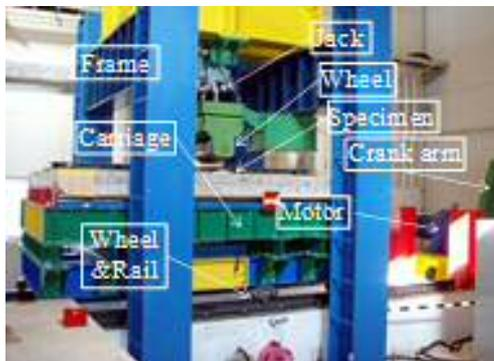
Fig. 1 Wheel tracking machine
